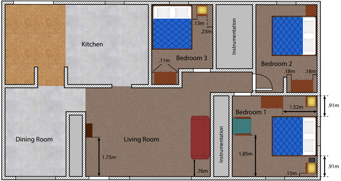
Figure 3.20: Plan view drawing of fuel configuration in the single story structure for bedroom 1 fires.
