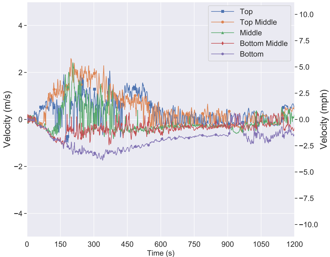
Figure 4.64: Experiment 9, no exterior ventilation openings, hallway velocity versus time. Positive velocity flowing from bedroom to living room.
