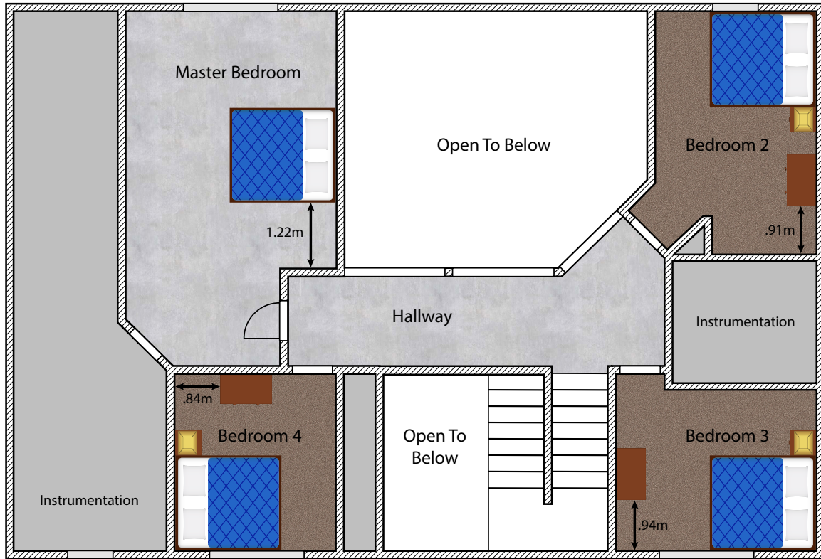
Figure 3.25: Plan view drawing of fuel configuration in the second floor of the two story structure.
