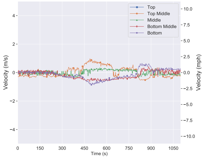
Figure 4.36: Experiment 6, no exterior ventilation openings, hallway velocity versus time. Positive pressure flowing from kitchen/living room to bedroom 2.
