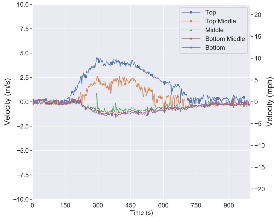
Figure 4.76: Experiment 13, front door and bedroom 1 windows open, front door velocity versus time.
